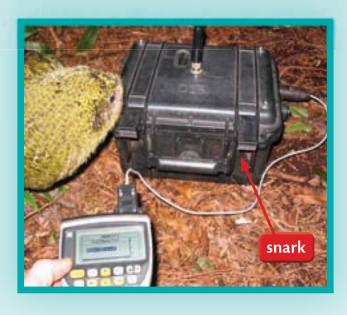
Another helpful tool is called a **snark**. The snark is a box with a radio **receiver** and a small computer inside. Scientists have placed snarks all around the island. The snarks pick up the birds' signals when they are on the move. Like the backpacks, the snarks help the recovery team know where to find the kakapo.
